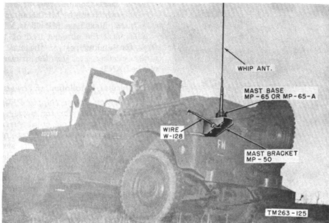
Figure 39. Typical installation of vehicular antenna.
