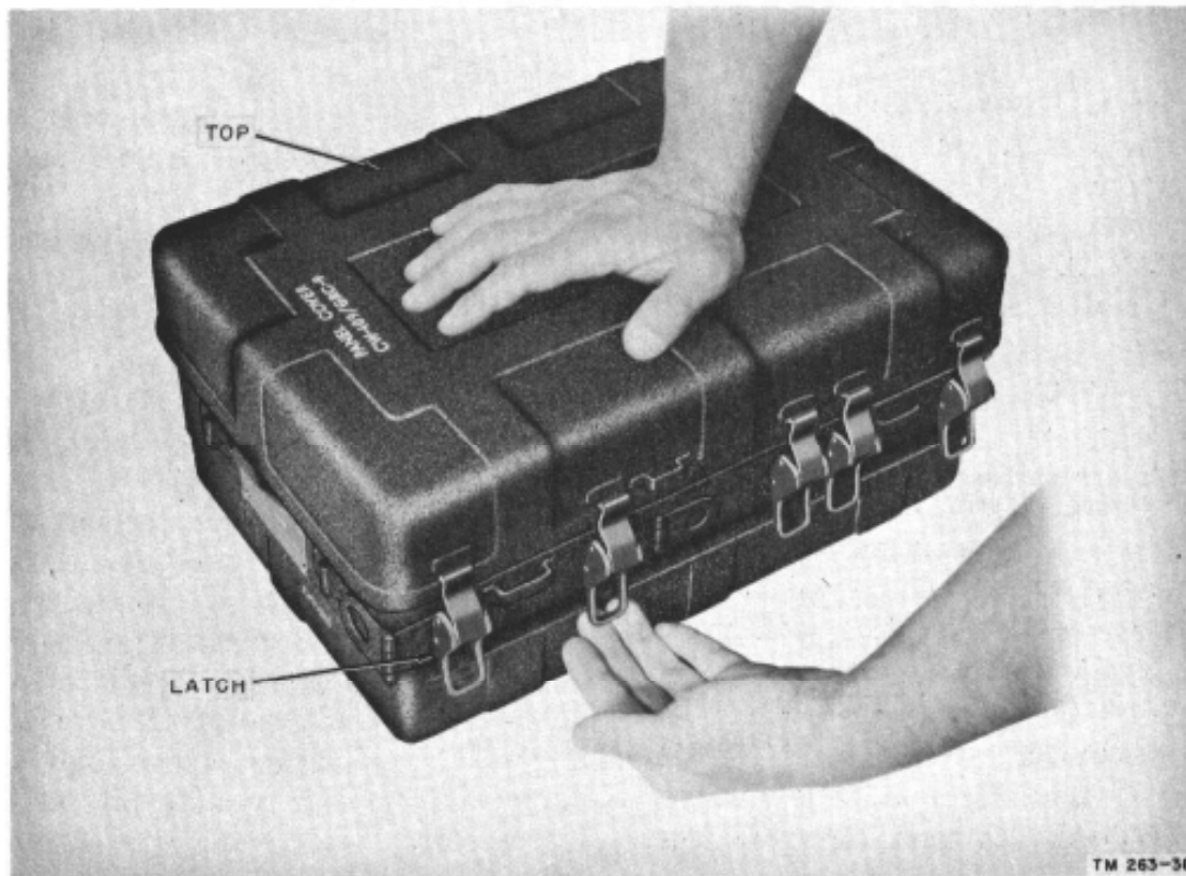
Figure 28. Removing front cover of receiver-transmitter.
